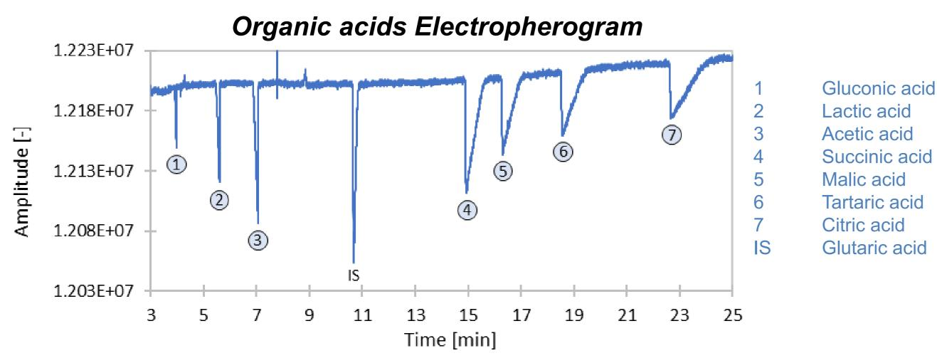
Conditions : BGE PDC (2,6-pyridinedicarboxylique acid) 15 mM pH 8.8, 20 kV, hydrodynamic injection (50 mbar, 8 s), indirect UV detection (255 nm)
