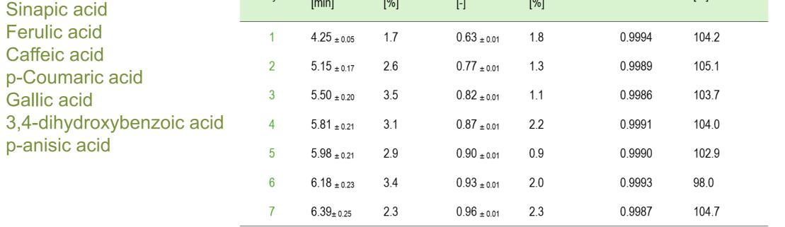
Conditions : BGE phosphate 50 mM pH 8.5, 10 kV, hydrodynamic injection (50 mbar, 8 s), direct UV detection (255 nm)
