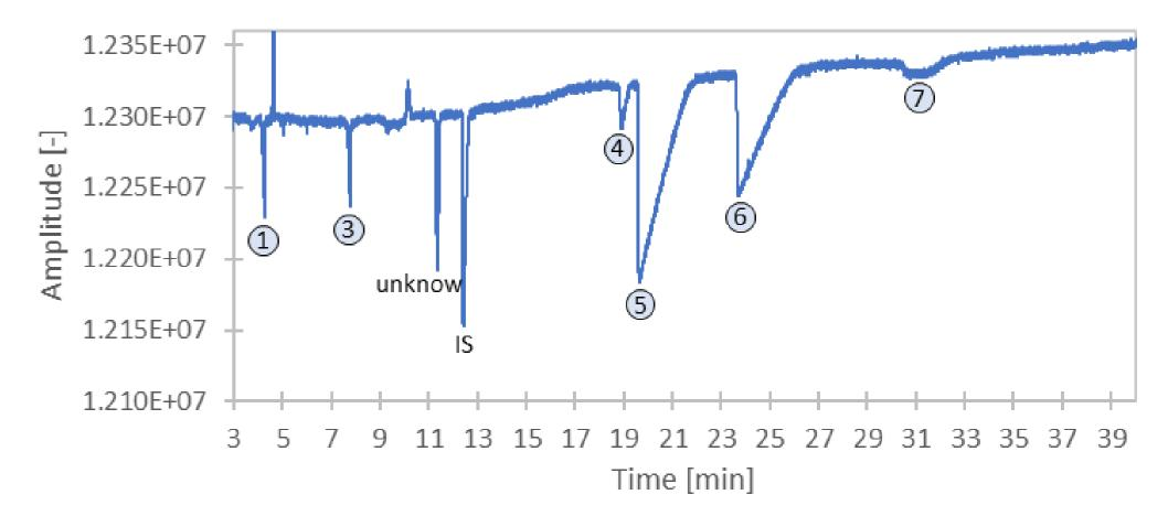
Conditions : BGE PDC (2,6-pyridinedicarboxylique acid) 15 mM pH 8.8, 20 kV, hydrodynamic injection (50 mbar, 8 s), indirect UV detection (255 nm)
