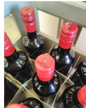
A serie of bottles sampled from each filling head during audit #2 in order to confirm the quality of the maintenance completed of the bottling line prior to the audit
