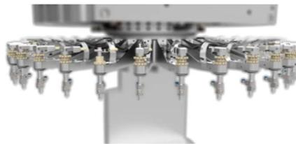
Rotating Turret equipped with 20 or 32 Pickup heads (PUH)
